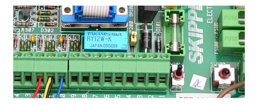
GDS101 Terminal board will normally not be supplied with pins for jumper and will need soldering.
